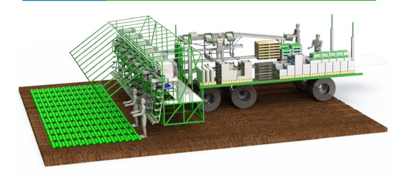
The Atlantis harvesting header system is the packing solution based on conventional / traditional harvesting systems, and can easily be used on fields with different planting concepts. The cutters can be assigned freely (within limits) to the different in-feed systems, and iceberg rows. The Atlantis header system itself can be operated in both harvesting directions, forward and
